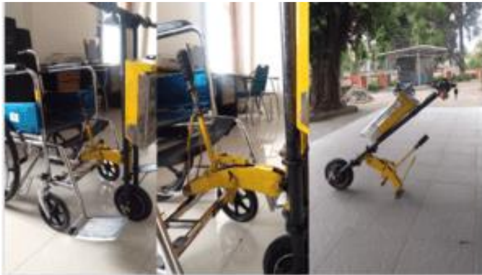
Gambar 3. Prototipe-1 Detachable Electric Drive for Wheelchair [Sumber: [5] ]
