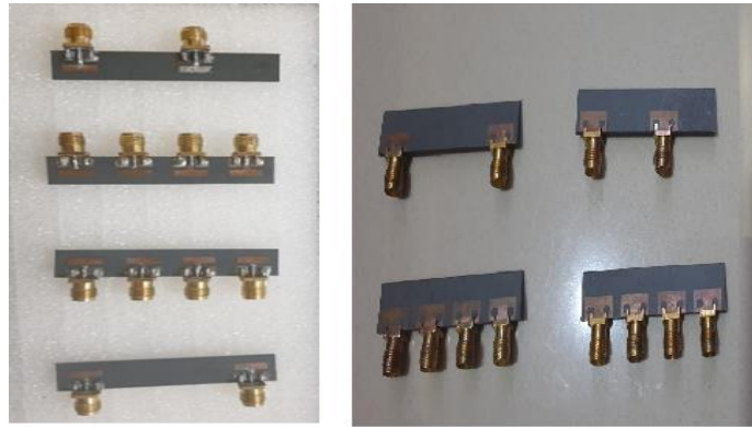
Fig. 9. Antennas After Fabrication
