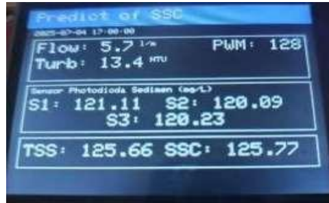
Figure 14. LCD Display Showing Realtime SSC Monitoring
