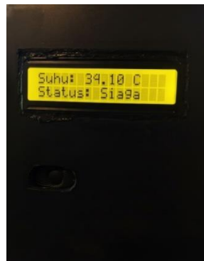
Gambar 6. Tampilan LCD Suhu 34,10°C Status Siaga
