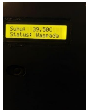
Gambar 7. Tampilan LCD Suhu 39,50°C Status Waspada
