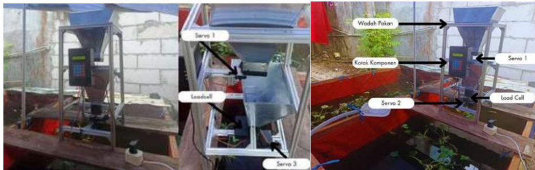
Figure 3. Final design implementation of the smart auto feeder.
