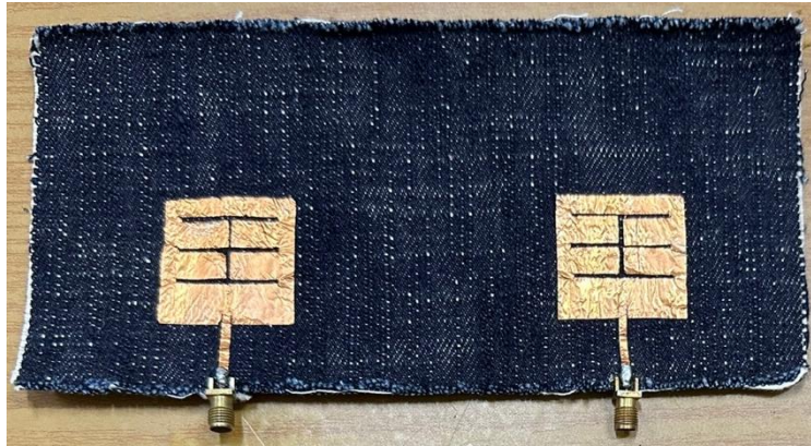
Figure 3. The fabricated of denim jeans-based textile MIMO antenna with slot.
