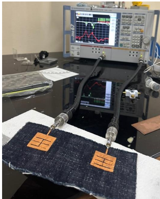
Figure 4. Measurement setup for denim-based textile MIMO antenna with slot.
