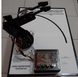
Gambar 28 Prototype Robot Manipulator 4 DOF Berbasis Raspberry Pi Zero W
