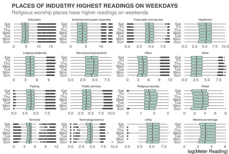
Figure 9. For each building's utility, record readings within a week.
