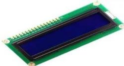
Gambar 5. LCD 16x2
